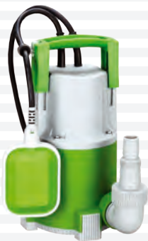
Submersible pump / Potopna pumpa AGRINA Q750124 750W; 8.5m; 7m; 0.85bar; 12500l/h; 23.5kg
