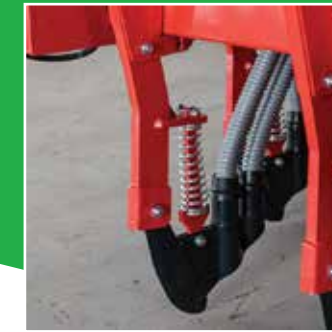
Spring loaded axe-type coultters perform best soil dipping.
