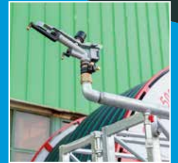
The sprinkler (Mariner from Italy) on the wing increases the irrigation distance.
