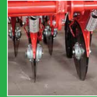
The discs are designed to use them in the cases where there is plenty of straw in the field.
