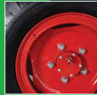
This pin is used for to disconnect the wheels from the gearbox and access to transportation mode.
