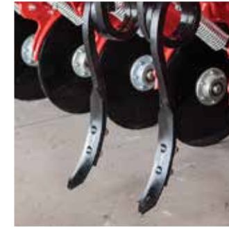
The cultivator legs fluff the soil out for a successful sowing operation.
