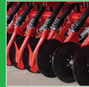
The sowing discs are durable and strong for the tough soil conditions.
