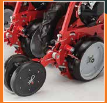
The pressure wheels which are behind the discs provide best seed covering and protect humidity in the soil.
