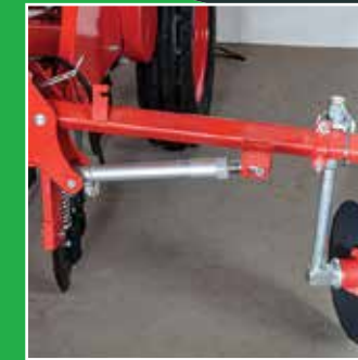
To open and close the markers will take just seconds with hydraulic support.
