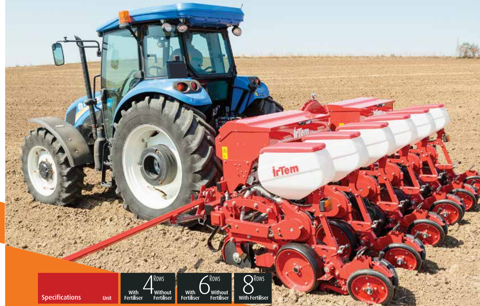
The pressure wheels which are behind the discs provide best seed covering and protect humidity in the soil.
